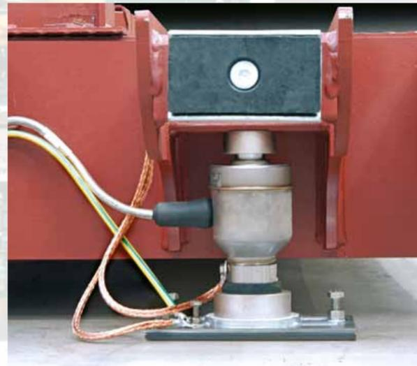
The calibration data for each load cell in the digital version are **memorised in the electronic memory**, thus **facilitating** calibration, the search for faults, maintenance and repair.
